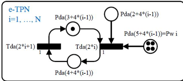
Fig. 2. e-TPN model for an elementary assembly operation
