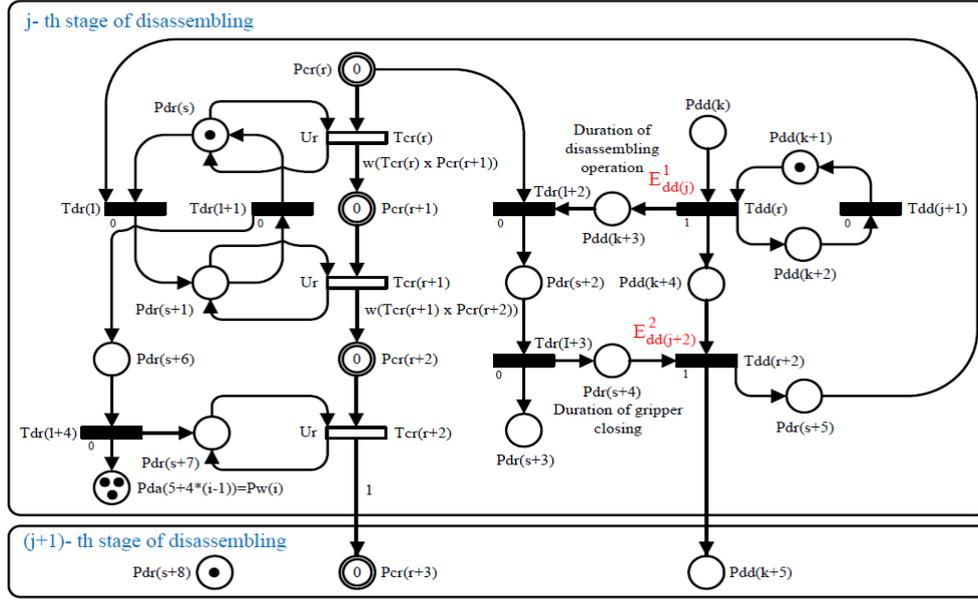
Fig. 3. e-SHPN model corresponding of j-th elementary disassembly operation
