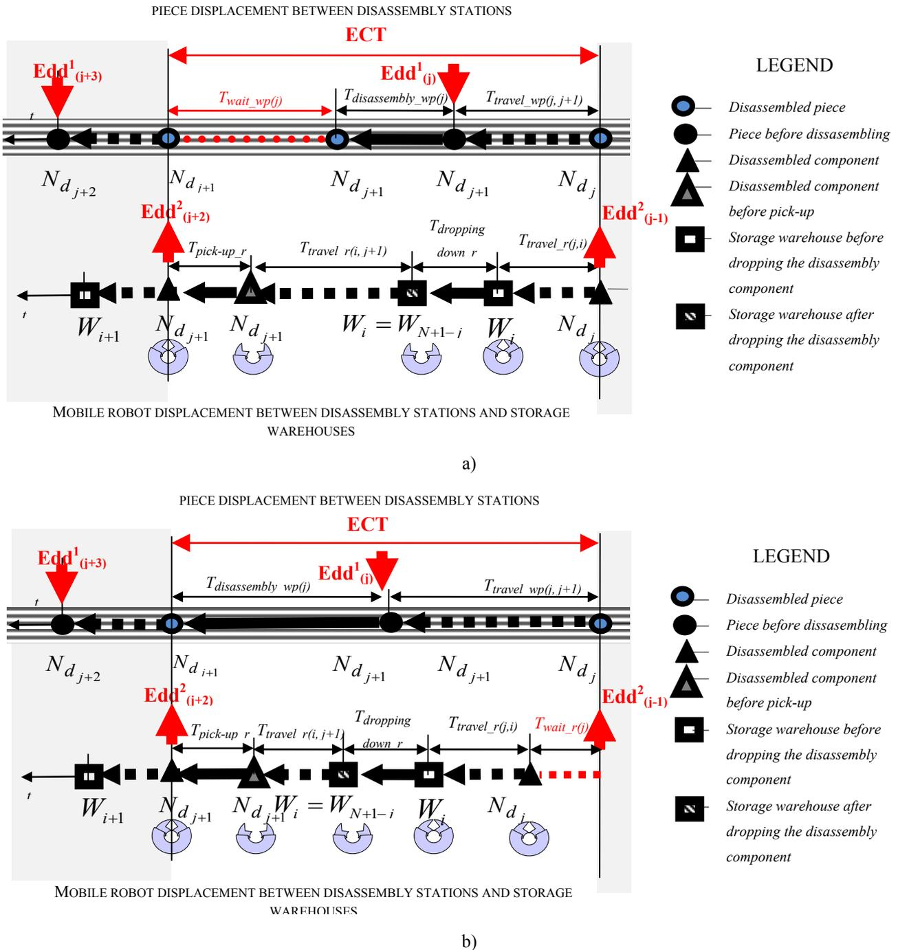
Fig. 6. Time intervals during elementary sequence of disassembly for a)  $ECT_R > ECT_{WP}$  ; b)  $ECT_R < ECT_{WP}$
