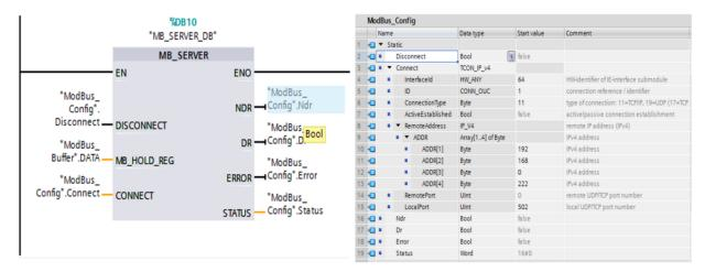
Figure 16. Siemens Modbus Server configuration in main routine.
