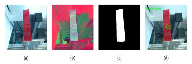
Figure 22. Warehouse reference color detection: (a) raw RGB image, (b) BGR to HSV conversion, (c) HSV limits are imposed and the result is shown as a white blob with a black background, (d) the reference color is detected, and the centroid is tracked.
