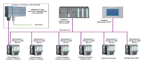
Figure 12. PLC hardware structure of the Mechatronics line Hera&Horstmann.
