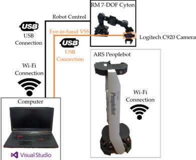
**Figure 14.** Communication block set of the computer between the FC, ARS PeopleBot WMR equipped with the Cyton RM and *eye-in-hand* VSS.
