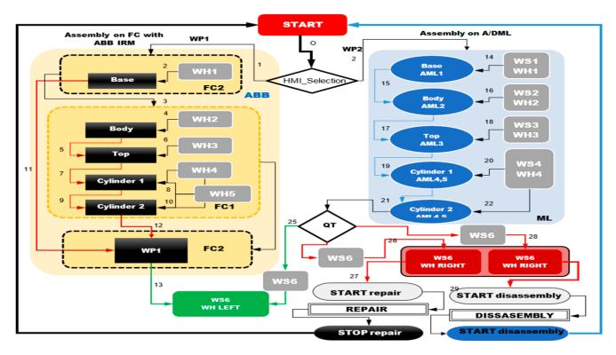
Figure 9. Task scheduling for assembly functionality.
