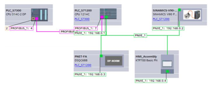
Figure 2. Flexible Cell Siemens S7-1200 PLC hardware structure.
