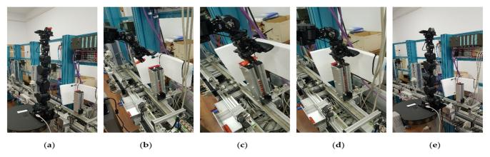
**Figure 21.** Real-time control of the RM Cyton located at the cylinders warehouse which has the resulting actions: (a) parking position with the object in the gripper, (b) scanning position, (c) moving above the warehouse, (d) placing the piece in the depot, (e) returning to home position.
