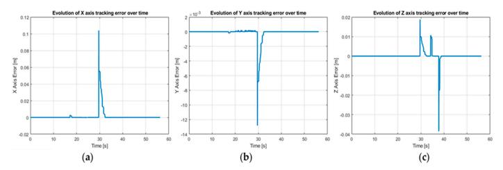
Figure 26. Tracking errors for RM Cyton picking object trajectory on: (a) X axis, (b), Y axis, (c) Z axis.
