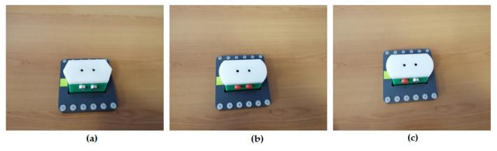
**Figure 7.** Assembled workpieces: (a) workpiece with metal cylinders; (b) workpiece with plastic cylinders; (c) workpiece with different material cylinders.
