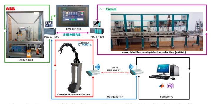
**Figure 1.** Control structure of A/DML Hera&Horstmann, FC with ABB IRM and CAS with PeopleBot WMR and Cyton 1500 RM.
