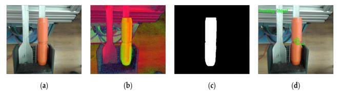
Figure 20. Object Detection with the following steps: (a) raw RGB image taken from the camera, (b) conversion from BGR to HSV (c) image segmentation after HSV limits are set, with morphological operations of erosion and dilation, (d) object is detected and the centroid is being tracked.
