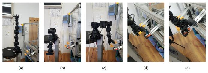
**Figure 18.** Real-time control of the 7-DOF Cyton 1500 RM located at the FC with the following sequences: (a) home position, (b) intermediary position, (c,d) scanning position, (e) picking object.
