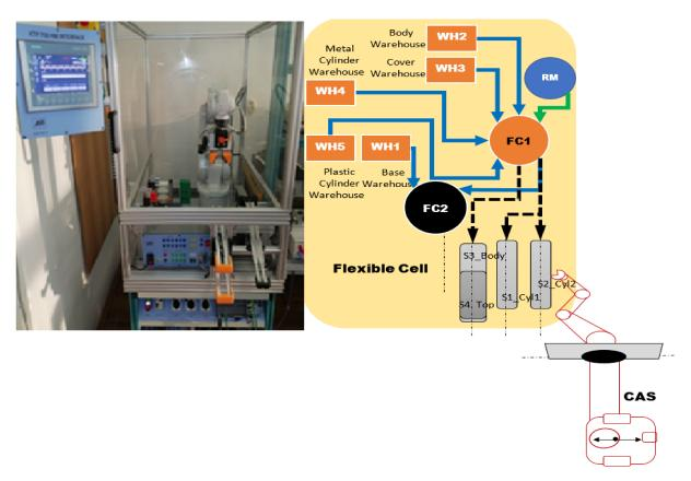
Figure 3. Flexible Cell Station with 6-DOF ABB IRB120.
